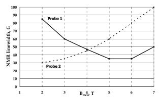
Fig. 2: Dependence of the resonance linewidth upon the Wiggler field value in the median plane.
