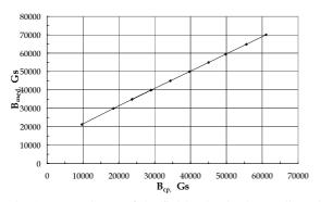
Fig. 3: Dependence of the field value in the median plane  $B_{med}$  upon the field value in the central pole  $B_{cp}$ .
