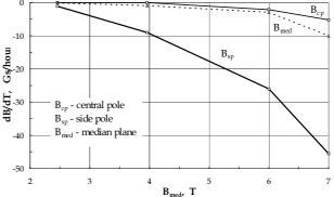
Fig. 5: Dependence of the rate of field degradation on the wiggler field value.
