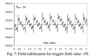
A current pumping operation has a consequence of the field ripples with the amplitude of  $0.5\div0.7$  Gs at the
