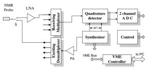
Fig. 4: A simplified scheme of the NMR System. PA - power amplifier, LNA - low noise amplifier, S - receiving/exciting switch.
