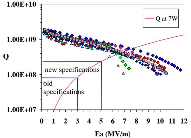
Figure 2: Rf test results of the 80 MHz, low- $\beta$  superconducting cavities. Only cavity n. 8 (square marker) underwent high pressure rinsing.
