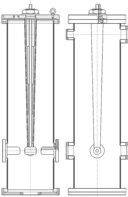
Figure 5: Schematic drawing of the 80 MHz rebunchers.
