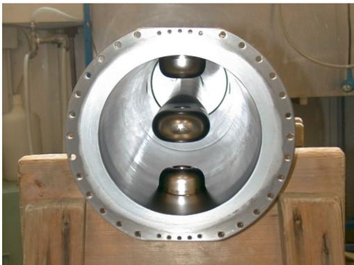
Figure 1: View of a PIAVE type bulk niobium cavity.
