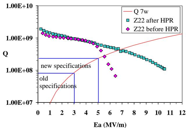
Figure 3: Effect of high pressure water rinsing in the last cavity tested.
