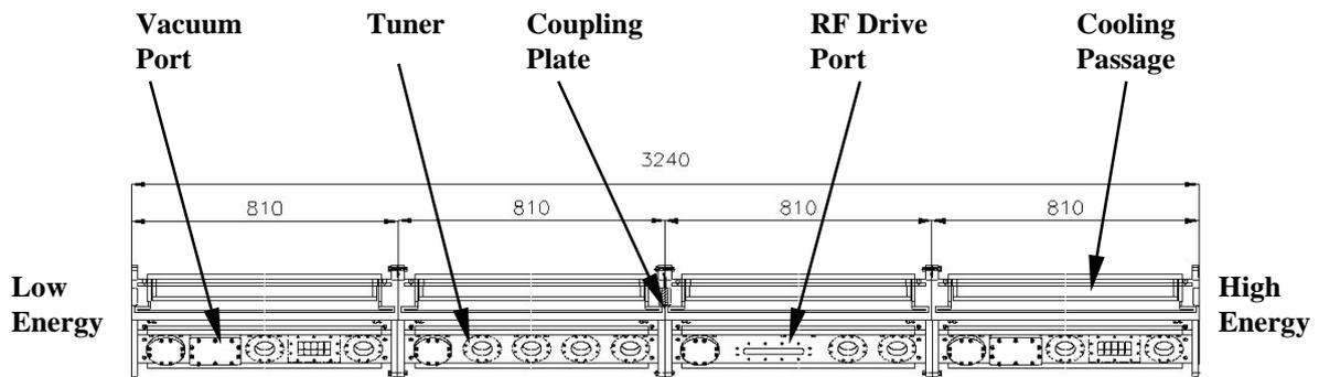
Figure 1. 3MeV, 350MHz, cw KOMAC/KTF RFQ
