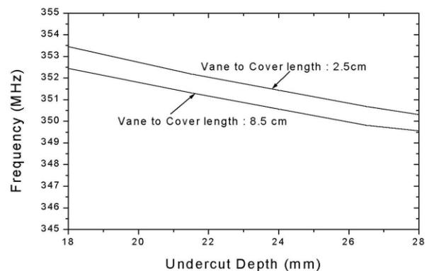
resonant frequency versus a depth of undercut.
