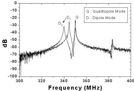
Figure 5. A shift of a dipole mode by a stabilizer rod:
