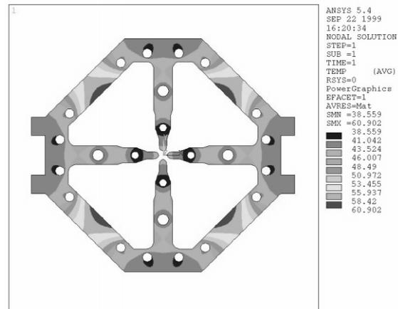
Figure 3. Temperature distribution of the cavity at the high energy end of the 0.45MeV RFQ.
