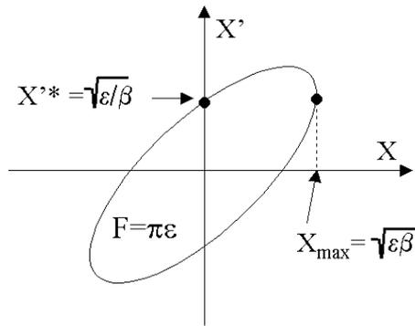
Figure 3: Measured emittance parameters of the beam.
