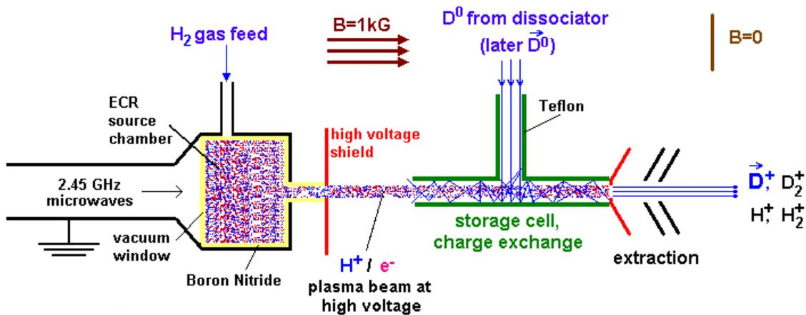
Figure 1: Scheme of the new polarized ion source.
