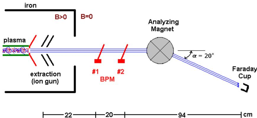
Figure 2: Accelerated beam diagnostic systems.
