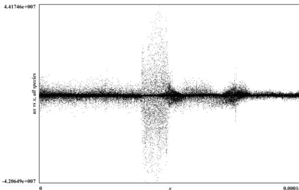
Figure 5: Snapshot of electrons in phase-space after the injection pulses collide.
