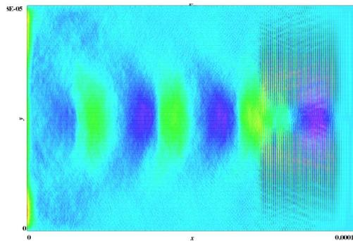
Figure 1: Longitudinal electric field as a function of distance
