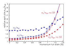
Figure 4: Relative rms spot sizes as a function of the fullwidth energy spread for a flat distribution with and without synchrotron radiation. The ideal linear spot sizes are  $\sigma_{x0} =$ 43 nm and  $\sigma_{y0} = 1.0$  nm.
