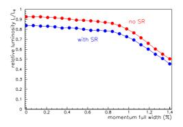
Figure 3: Relative luminosity loss as a function of the fullwidth energy spread for a flat distribution. The luminosity was calculated by tracking two random distributions of 5000 particles through the final focus to the IP and there convoluting them on a grid. The ideal reference luminosity without pinch is  $L_0 = 4.6 \times 10^{34} \text{ cm}^{-2} \text{s}^{-1}$ .
