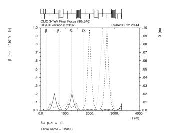
Figure 1: Beta functions and dispersion for the entire finalfocus system as a function of the longitudinal position. The interaction point is on the right.
