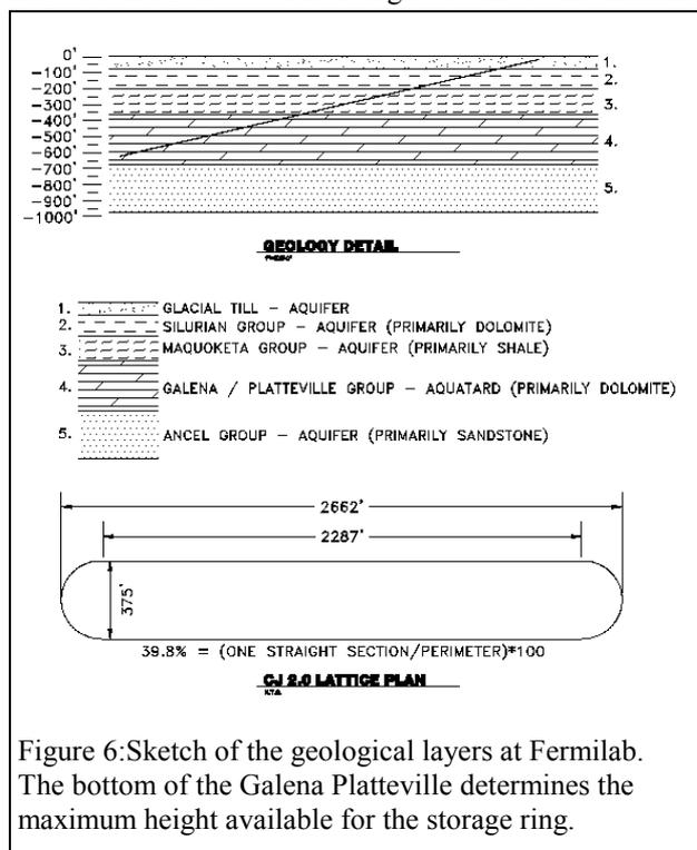
Figure 6: Sketch of the geological layers at Fermilab. The bottom of the Galena Platteville determines the maximum height available for the storage ring.
