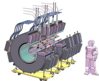
Figure 3: Sketch of an induction cell with integrated sc 3 T coils.
