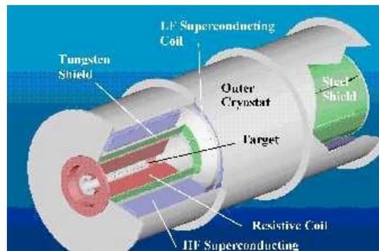
Figure 2: Target insert with sc coil and normal conducting 10 T insert.
