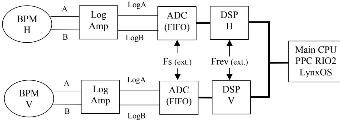
Figure 3: The hardware proposed for the large oscillation interlock
