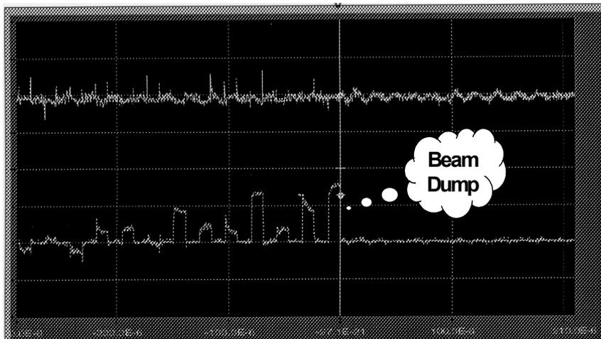
Figure 2: An actual beam-dump from the present large-position interlock system as seen using a digital storage oscilloscope.
