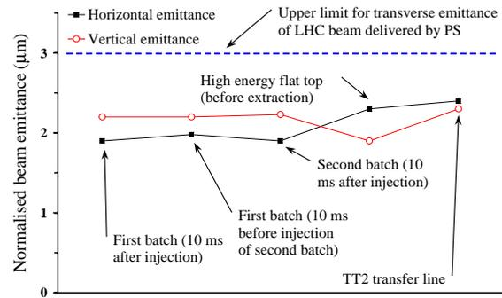
Figure 3: Evolution of the normalised transverse beam emittances  $\varepsilon_{x,y}^*$  from PS injection to TT2 extraction line.
