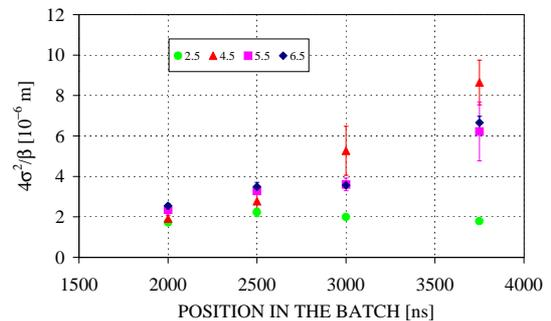
Figure 1: Horizontal profile measurement along the batch a few ms after injection for different batch intensities (expressed in  $10^{12}$  p)
