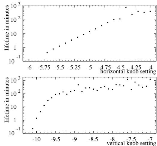
Figure 1: Results of vertical scraping measurements in the HER with single beams. The top plot shows the horizontal, the bottom plot the vertical plane. The knob setting is given in mm at the collimator. Moving in the negative direction on the knob brings the beam closer to the collimator.
