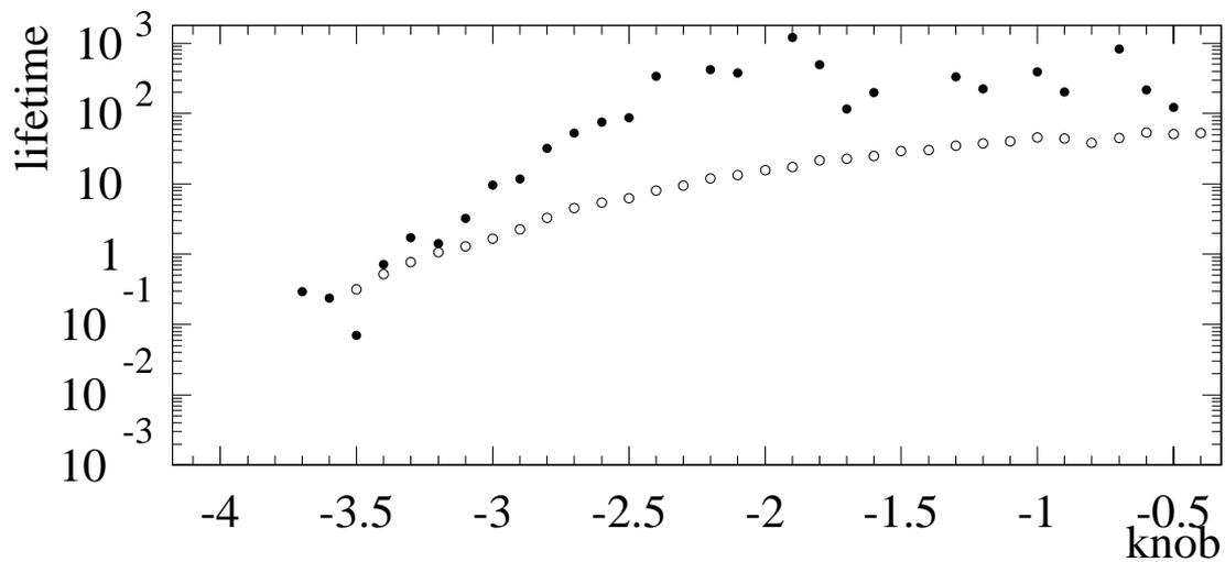
Figure 3: Results of horizontal scraping measurements in the LER with colliding beams. Open circles are with high, bullets with low currents. The knob setting is given in mm at the collimator and the lifetime in minutes. Moving in the negative direction on the knob brings the beam closer to the collimator.
