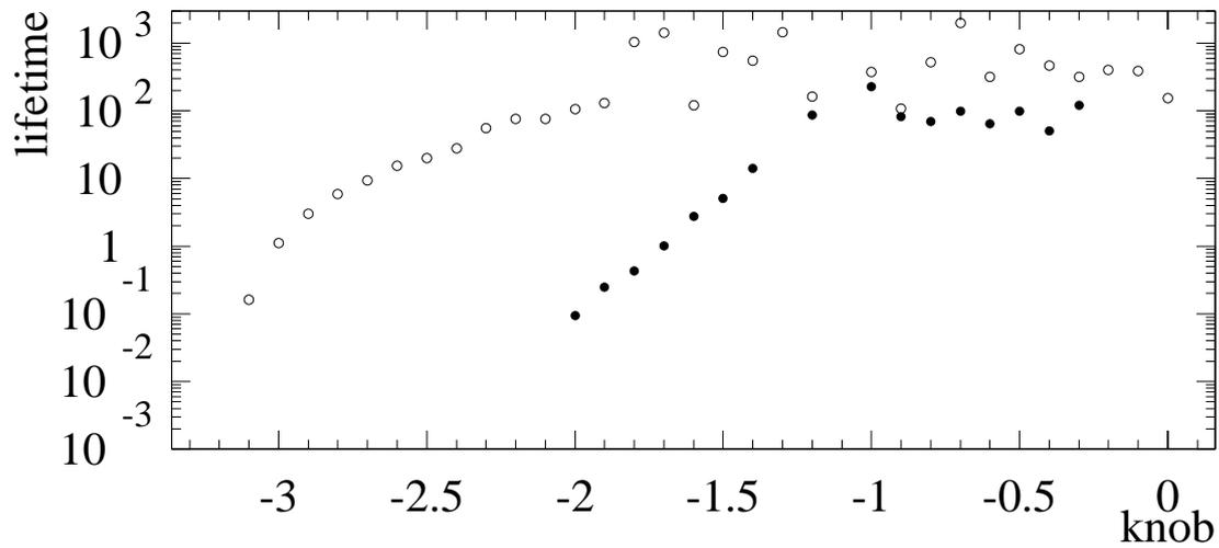
Figure 2: Results of vertical scraping measurements in the HER with colliding beams. Open circles are with high, bullets with low currents. The knob setting is given in mm at the collimator and the lifetime in minutes. Moving in the negative direction on the knob brings the beam closer to the collimator.
