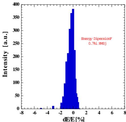
Fig.4 Energy distribution of electron bunches after the linac
