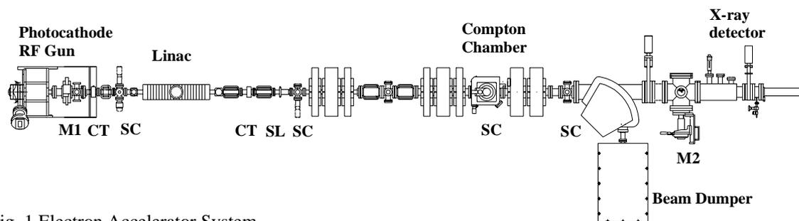
Fig. 1 Electron Accelerator System
