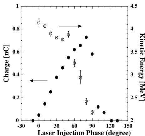
Fig.3 Charge and energy of electron bunches emitted from the gun vs. laser injection phase
