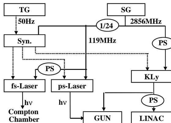
Fig.2 Block diagram of Synchronisation and RF system
