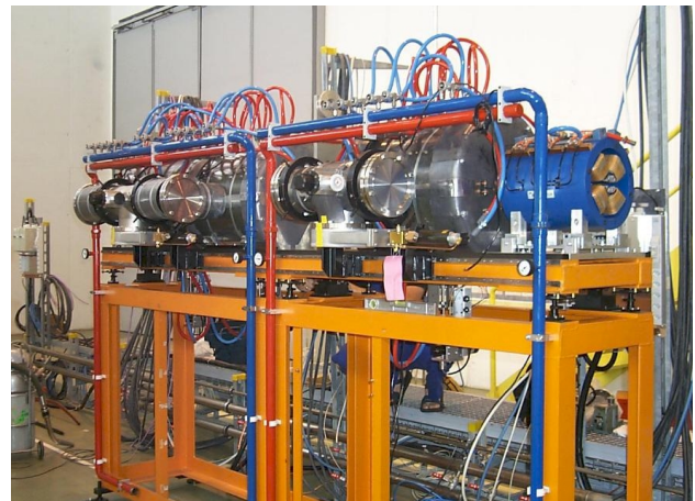
Figure 7: The 7-gap-resonator Linac mounted in the ISOLDE hall
