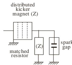
Figure 11: Spark-gap for decreasing the beam-coupling impedance
