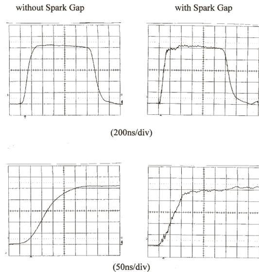
Figure 7: Effect of a spark-gap
