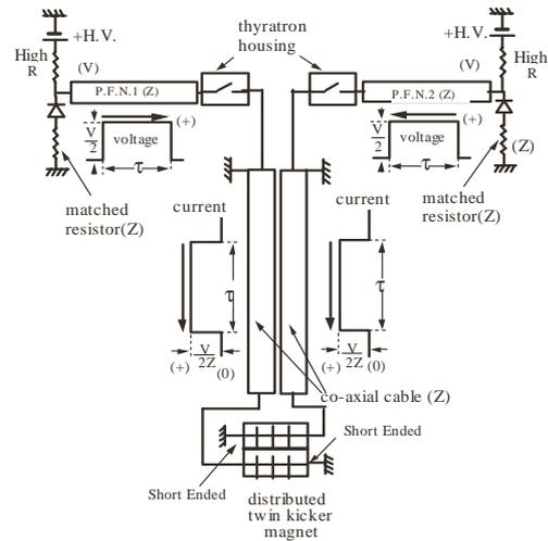
Figure 10: Separated power supply of the PFN potential with same the sign
