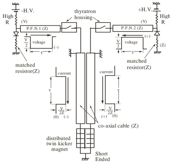
Figure 9: Separated power supply of the PFN potential with opposite the sign
