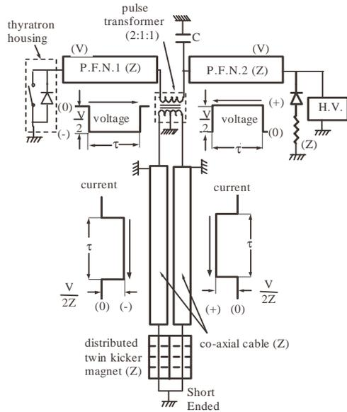
Figure 4: Blumlein system with a twin distributed kicker magnet
