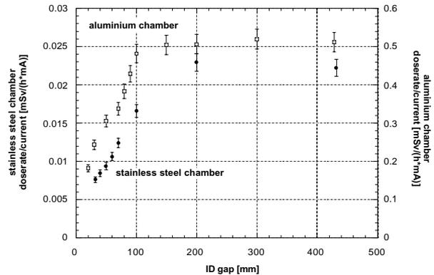
Fig. 6 - Doserate/current as a function of ID gap for the stainless steel and the aluminum chamber.
