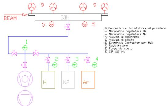
Fig. 1 - Experimental arrangement allowing gas injection into the ELETTRA storage ring
