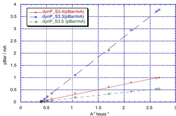
Fig. 3 - Dynamic pressures measured from the pumps at each side (circles, diamonds) and with a Penning head close to the center where gas injection occurs (squares).
