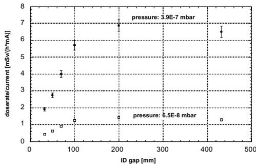
Fig. 5 - Normalized bremsstrahlung rate versus undulator gap with gas injection.
