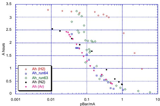
Fig. 2 – Product of lifetime and beam current as a function of local dynamic pressure
