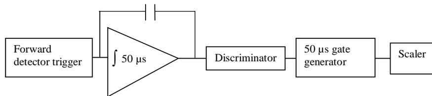
Fig. 3. To count the number of pellets which go through the CELSIUS beam, short (20 ns) logic pulses from the detector trigger is integrated with a time constant of 50  $\mu$ s. This corresponds to the expected time for a pellet to pass the beam. The discriminator selects pulse clusters of a certain size (see fig. 1), and the cluster rate is counted with a scaler. The signal for a cluster is prolonged to 50  $\mu$ s, to avoid double counting.
