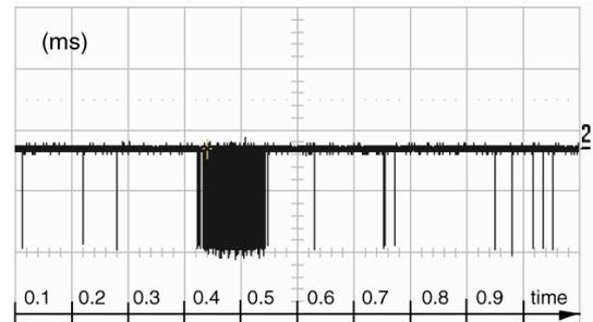
Figure 2. An oscilloscope trace showing the passage of a pellet through the CELSIUS beam. It shows pulses from single-track triggers in the forward detector.
