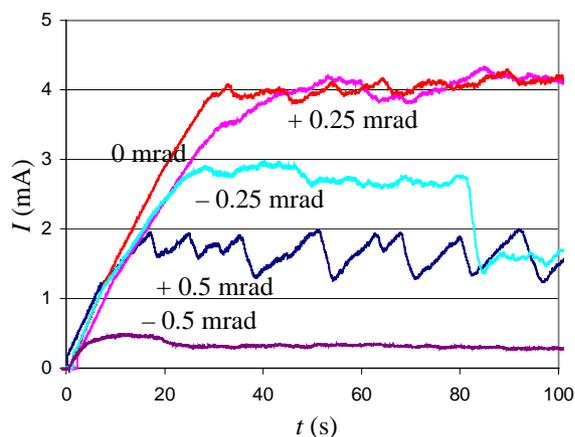
Figure 4. Accumulated ion current  $I$  as a function of time during stripping injection with cooling accumulation of 24.5 MeV/ $u$   $^{14}\text{N}^{7+}$  ions, done with different misalignment angles between the electron beam and the closed orbit.
