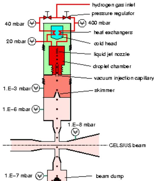
Figure 1. Schematic view of the pellet target system
