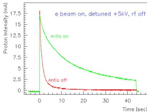
Figure 5. Plot of 48 MeV proton intensity vs. time with 100 mA electron beam current present in the electron cooler, with and without compensating for the electron cooler's magnetic field (0.1 T) with the antisolenoid.
