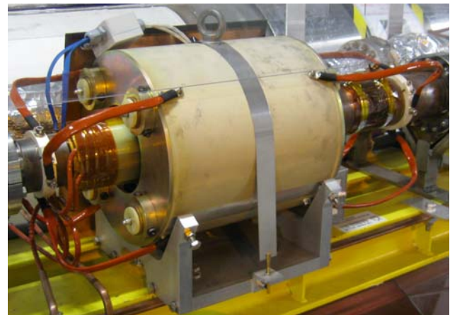
Figure 2: The DCCT with the connexions for the beam image current.
