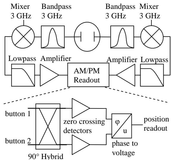
Figure 1: Block diagram of the BPM readout.
