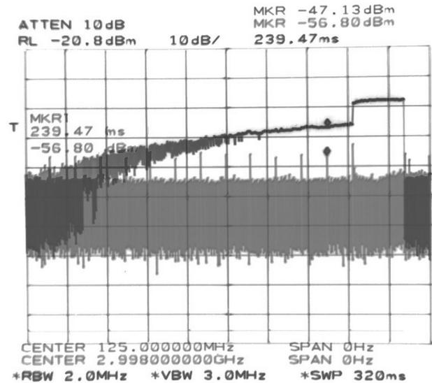
Figure 3: Frequency selected response of a single button, photographed from a spectrum analyzer in zero span mode. Two frequencies are shown, 125 MHz and 3 GHz.
