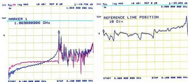
Figure 2: Frequency Response of the BPM.
