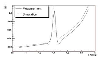
Figure 7: Transmission between orthogonal ports of at FLASH installed BPM without long cables: measurement and simulation (shift of slot position: 0.09 mm).
