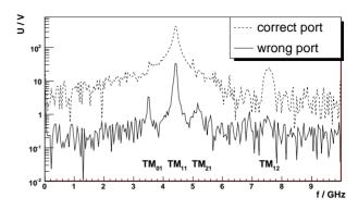
Figure 5: Fourier transformation of signals shown in Fig. 3. Monopole mode leakage at  $3.5\,\text{GHz}$  is observed too. The first quadrupole mode (TM $_{21}$ ) at  $5.2\,\text{GHz}$  and the second dipole mode (TM $_{12}$ ) at  $7.6\,\text{GHz}$  are visible.
