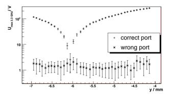
Figure 10: Maximum level at dipole resonance frequency of second prototype as a function of vertical mover position for both ports. Error bars are the standard deviation of several measurements. BPM center is at about -6.08 mm.
