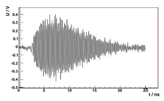
Figure 3: Time domain response signal of dipole resonator. Top: with beam offset of 1.08 mm, bottom: from the orthogonal port. Note the different vertical scales.
