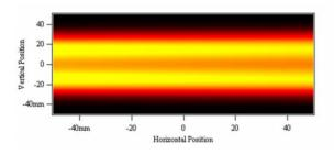
Figure 8: Simulation of the intensity distribution of the DA $\Phi$ NE bending magnet IR emission at the wavelength of 10  $\mu$ m.
