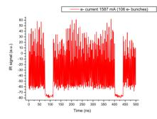
Figure 3: The DA $\Phi$ NE electron bunches structure as detected by a fast IR uncooled device.
