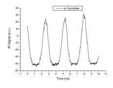
Figure 4: IR signal of three adjacent electron bunches.
