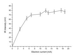
Figure 6: IR signal vs. the electron current.
