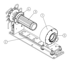
Figure 5: Mechanical design of the FBCTs used for the measurement in the LHC rings.
