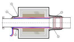
Figure 4: The sketch of the DCCT transformer.
