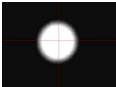
Figure 9 First beam at the Isocenter, measured with the isocenter-diagnostics device (beam diam.: 10 mm)
