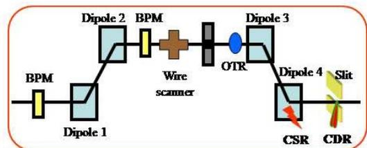
Figure 4: Magnetic chicane monitors at FERMI
