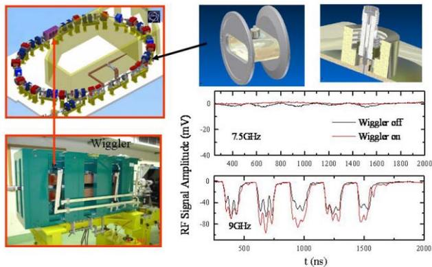
Figure 5: Bunch train combination in the Delay Loop
