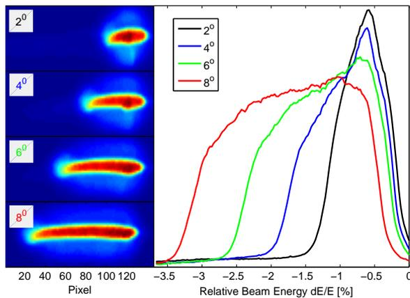
Figure 6: Transverse beam distributions and profiles for 4 off-crest acceleration phases of module ACC1.
