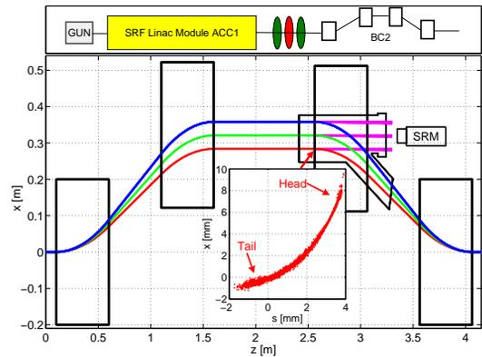
Figure 1: Top: Sketch of the FLASH injector. Bottom: Geometry of BC2 and beam trajectories for bend angles of 16°, 18° and 20°. Inset: Top view of particle distribution at 9° off-crest acceleration in module ACC1 (simulation).
