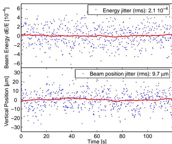
Figure 7: Single-bunch beam energy jitter measured during a SASE run at  $9^\circ$  off-crest acceleration in module ACC1.
