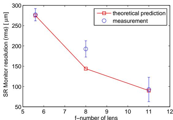
Figure 4: Resolution of SR monitor (for further explanation see text).
