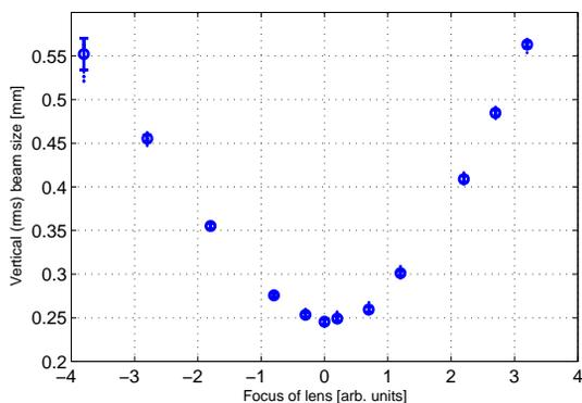
Figure 3: Measured rms beam size vs. lens focus.
