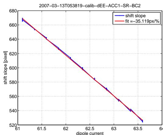
Figure 5: Energy calibration of SR monitor.
