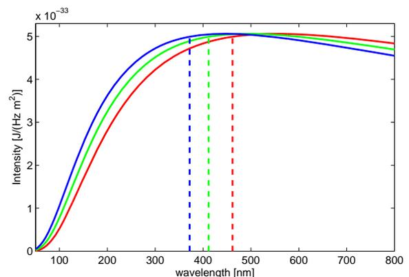
Figure 2: Spectral distribution of the SR calculated with Schwinger's equation for bend angles of 16°, 18° and 20° in BC2. Dashed lines indicate the corresponding critical wavelengths.
