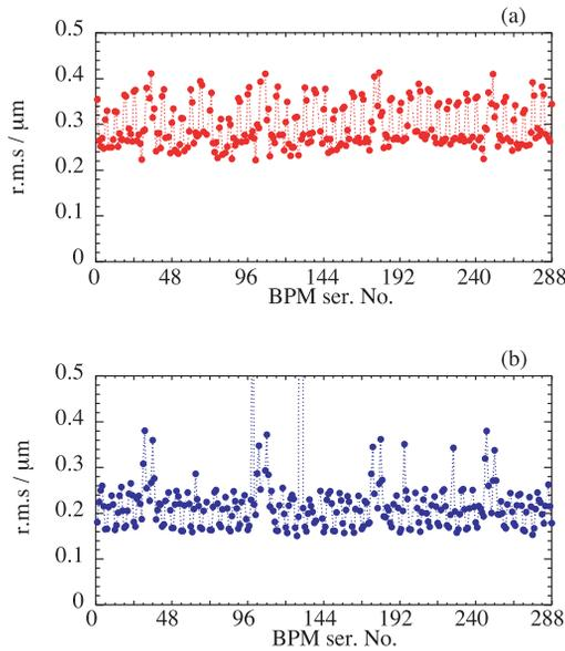
Figure 1: RMS values vs. BPM serial numbers. Lines just connect the points. (a):Horizontal, (b):Vertical direction. In the vertical direction, 2 points are out of the scale; they are 0.8  $\mu\text{m}$  at serial No. 99 and 1.9  $\mu\text{m}$  at serial No. 130.
