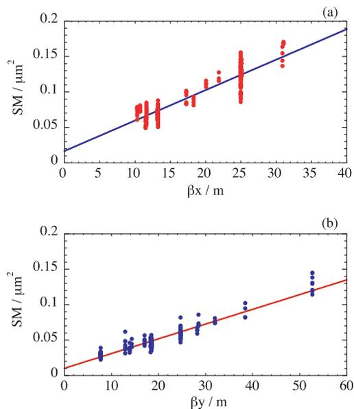
Figure 3: SM values vs. betatron function values at the corresponding BPM locations. The betatron function values are calculated ones with the lattice parameters of the optics for the operation condition. (a):Horizontal, (b):Vertical directions. The lines are the fitted ones with the equation (1). The parameters obtained by the fit are listed in Table 1.
