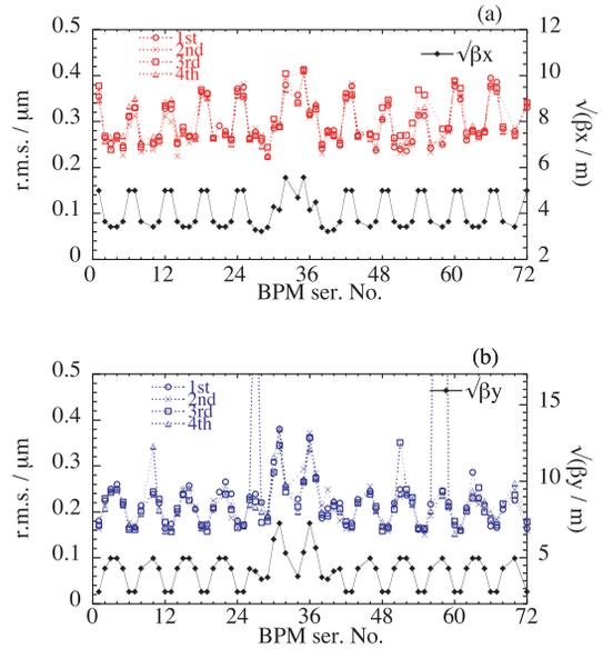
Figure 2: RMS values vs. BPM serial numbers for the left vertical axis. Square root of the betatron function values at the BPM locations are also plotted in black marks and lines for the right vertical axis. The points are translated by multiple of quadrant of the storage ring. (a): Horizontal, (b):Vertical direction. Open circle: first quadrant, cross: second quadrant, square: third quadrant, and triangle: fourth quadrant.
