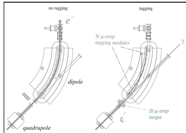
Figure 1: **Left:** layout of the final part of the BTF beam-line; the electron beam can exit either from the straight section (bending off), or from the  $45^\circ$  curved section (bending on). **Right:** layout of the photon tagging; the electron irradiates a bremsstrahlung photon on the silicon micro-strip target, and impinges on one of the 10 silicon micro-strip tagging modules outside the wall of the curved section of the beam-pipe.
