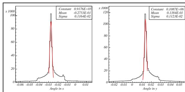
Figure 5: Horizontal and vertical angles of the electron tracks measured inside the target silicon micro-strip planes (energy of incoming electrons of 424 MeV).
