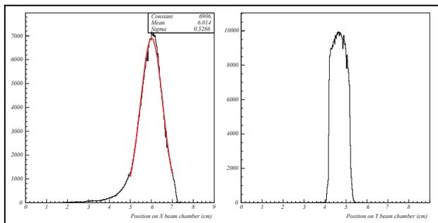
Figure 6: Impact point of the incoming electrons in the horizontal and vertical coordinates measured by the target silicon micro-strip planes (energy of incoming electrons of 424 MeV).
