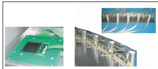
Figure 2: **Left:** silicon micro-strip chambers, acting as active target for bremsstrahlung; **right:** silicon micro-strip tagging modules.
