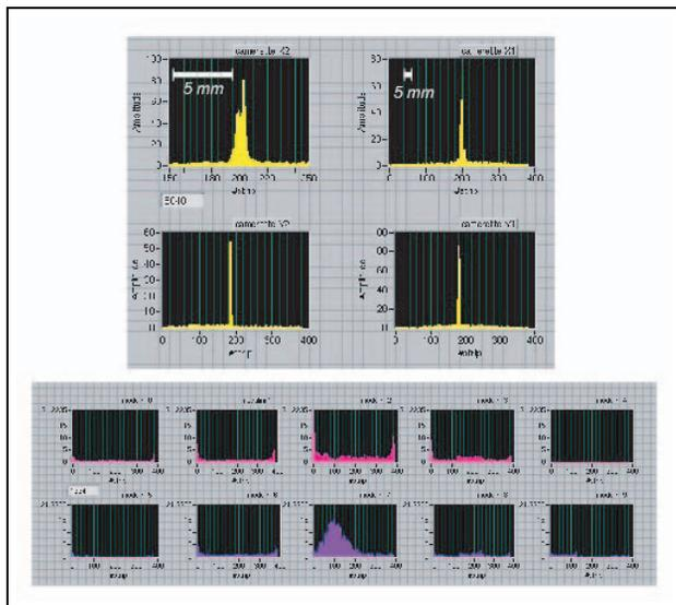
Figure 3: **top:** beam spot on the four silicon micro-strip chambers ( $x$ - $y$  views); **bottom:** electron beam on the silicon micro-strip tagging modules (divided in 2 supermodules, 5 detectors each) with magnetic field double with respect to nominal value.
