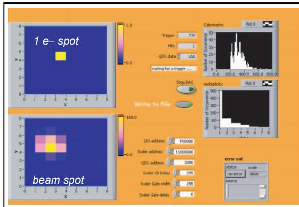
Figure 8: Online panel of the triple-GEM pads readout, showing the beam profile for one electron peak (top) or for the total beam spot (bottom).
