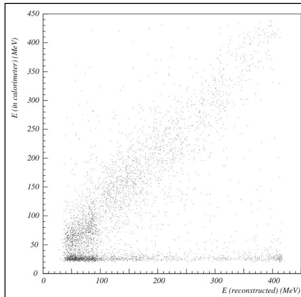
Figure 4: Energy of the photon measured by a calorimeter as a function of the energy reconstructed by the tagging system (energy of primary electrons of 424 MeV).
