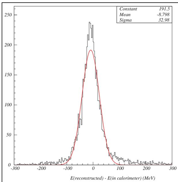
Figure 7: Difference between the photon measured by a test calorimeter and the energy reconstructed by the tagging system (energy of incoming electrons of 424 MeV).
