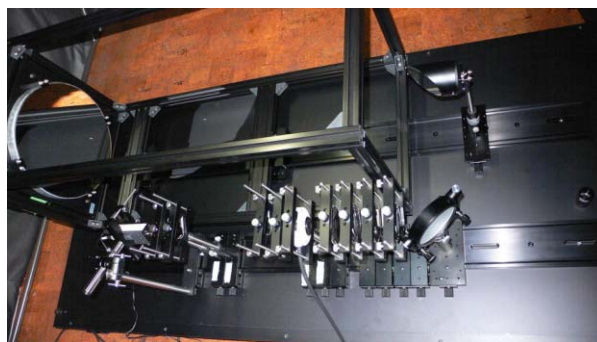
Figure 5: Newly-developed optical system using a Newtonian reflecting telescope.
