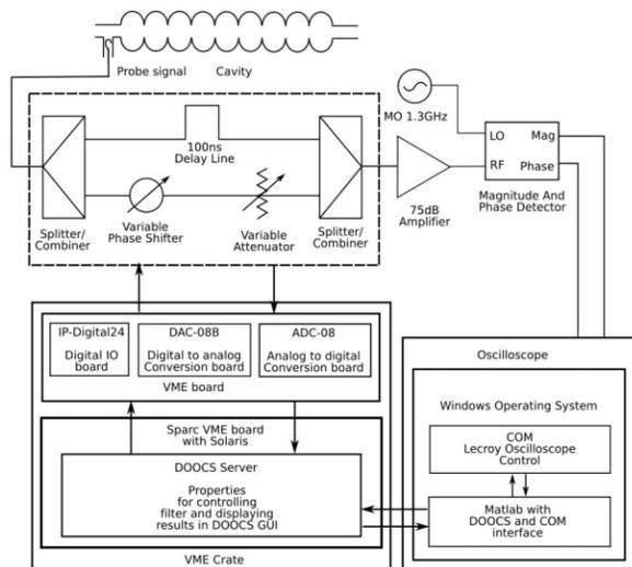
Fig. 5 Block diagram of automatic adjustment circuit
