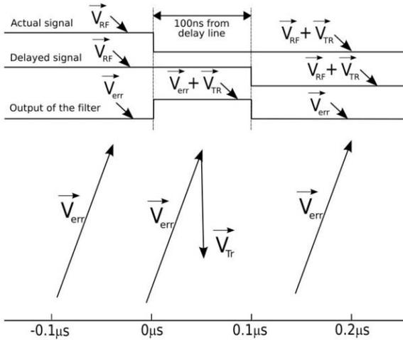
Fig. 2 Subtraction of delayed signal from actual signal
