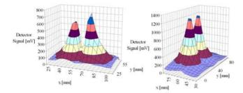
Figure 5: Intensity distribution of the horizontal (left) and vertical (right) polarization of CTR, measured at the SLS LINAC (set-up A). The asymmetry in the horizontal scan is predicted by the model when considering the target screen to be rotated by 45 degree into the electron beam.
