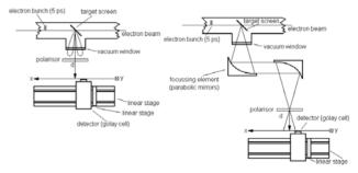
Figure 4: Set-up A (left): Mapping of the CTR farfield at a distance d of 250 mm from the source. Setup B (right): Two parabolic mirrors with focal lengths of 200 mm and 60 mm diameter were used to produce an image of the source. The CTR intensity distribution was then measured at a distance of 70 mm from the focal plane.
