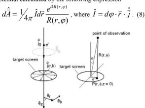
Figure 2: Left side: the magnetic field inducing currents. Right side: observation of radiation in the farfield.
