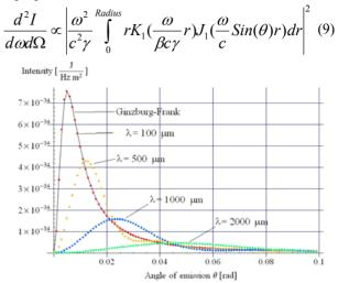
Figure 3: Emission characteristic of CTR for a single electron with normal incidence on a circular target screen of radius 19 mm. For wavelengths of  $< 100 \mu m$  the characteristic agrees well with the expression (5) given by Ginzburg and Frank.
