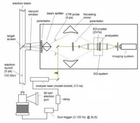
Figure 1: Schematic setup for EO-auto-correlation.
