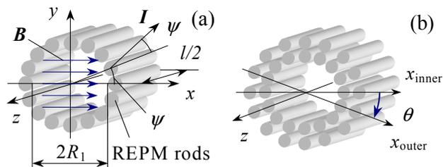
Figure 3: Rod type dipole – (a) and (b) – field compensation method in two-layer construction.
