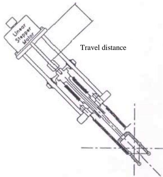
Figure (1) Schematic view of the wire scanner.
