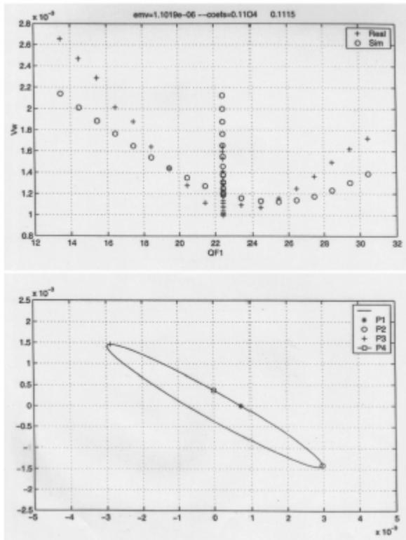
Figure (4) Width of vertical profile versus current of QF1 and simulation fitting, and the ellips correspond to the emittance
