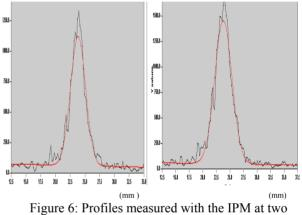
Figure 6: Profiles measured with the IPM at two different gains of the same coasting beam of 2  $10^{12}$  p.
