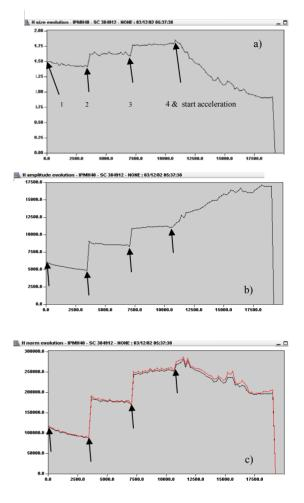
Figure 4: Evolution of: a) the horizontal beam rms, b) the amplitude and c) the integral of the IPM signal during injection then acceleration of 4 batches of 72 bunches of  $1.1 \ 10^{11}$  protons.
