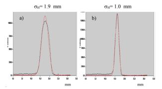
Figure 3: Profile of beam prepared for the LHC: 288 bunches of  $1.1 \ 10^{11}$  protons: a) before (26 GeV) - b) at the end of acceleration (450 GeV).
