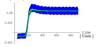
Fig 1. Blue curve: Filtered PLL output. Green curve: Same PLL but with improved filter put onto the phase detector.
