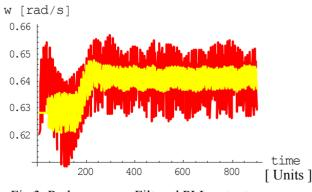
Fig 3. Red curve: Filtered PLL output. Yellow curve: Same PLL but with improved filter put onto the phase detector.
