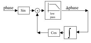
We can now introduce the concept of "phase detector" and VCO (Voltage controlled Oscillator):
