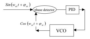
When the PLL is locked, the two inputs of the phase detector are 90  $^{\circ}$  out of phase or "in quadrature".
