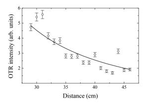
Figure 5: OTR intensity versus distance from the screen.
