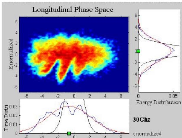
Figure 1: simulation of a microwave longitudinal instability caused by a 30 GHz broadband impedance [1]
