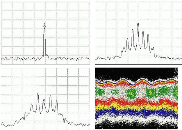
Figure 5a, b, c, d: Spectrums of the  $\Sigma$  signal detected on the 16.2 GHz cavity at 5mA, 10mA, 16mA in single bunch (scale 10 KHz/div-10dB/div) and streak camera image at 16mA (scale: 1000 turns X 150ps).
