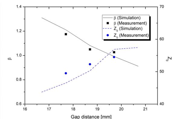
Figure 7. Results of RF coupling coefficient and characteristics impedance
