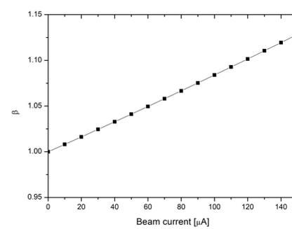
Figure 3. Calculation result of RF coupling coefficient according to beam current
