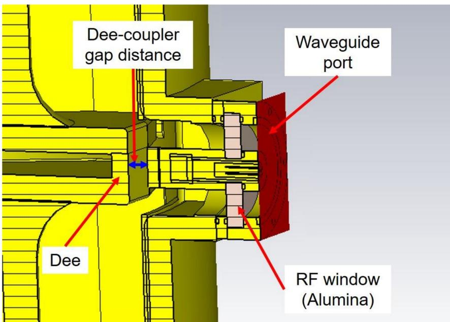
Figure 2. Scheme of power coupler
