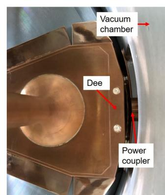
Figure 6. Dee and power coupler in SKKUCY-10 RF cavity
