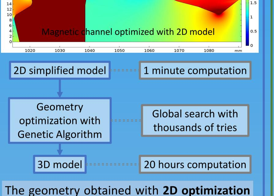
is able to produce the same amount of gradient when used in the 3D model, but the uniformity obtained with the 2D optimization is no more valid in 3D model.
