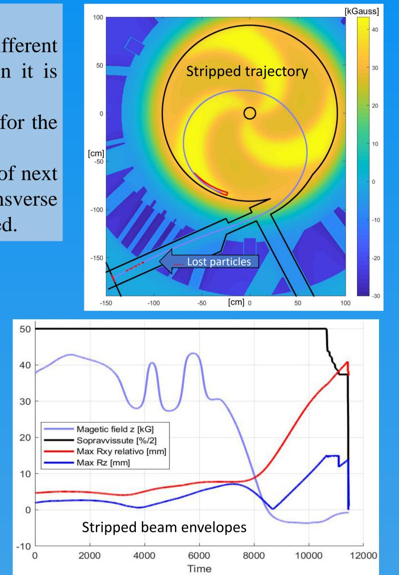
In correspondence of the escape from acceleration region, a strong defocusing is observed for the envelope in the middle plane, while strong focusing occur in the vertical direction. The result is that after the cyclotron the envelope of the beam is bigger than the acceptance of next set of quadrupoles. Further disagreement with respect next optical requirement is that the transverse and the vertical envelope of the beam are not one convergent and the other divergent as needed.
