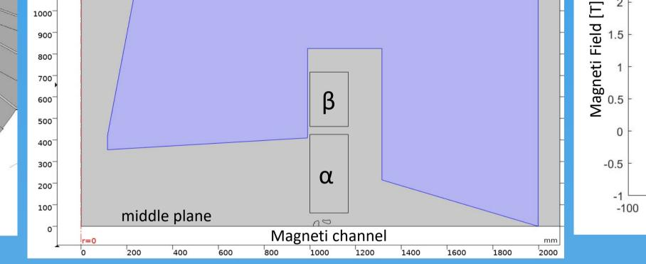
The geometry obtained with **2D optimization in a 3D-equivalent environment** produces the same gradient when applied in the 3D model. Magnetic field gradient uniformity is confirmed and excellent result of genetic algorithm approach is preserved.
