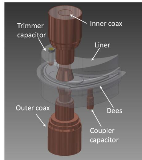
Figure 3: 3D model of RF cavity of the cyclotron.
