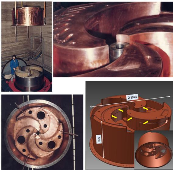
Figure 4: Liner assembling phases, about 30 years ago, the yellow arrows show the possible vacuum leakages in the welding points between vertical and horizontal wall.
