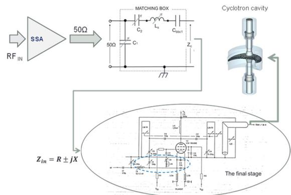
Figure 5: Block diagram of the refurbished amplifier.
