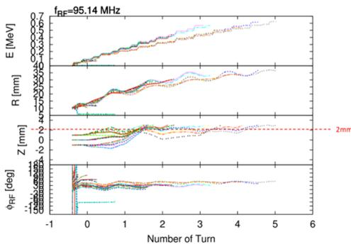
Figure 5: Parameters of deflected beam orbit till the beam dumps.
