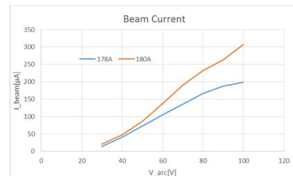
Figure 3: Extracted beam current on the test bench. This shows arc voltage vs extracted beam current in case of two type of filament current.
