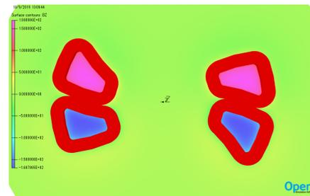
Figure 7: Bz 1<sup>st</sup> harmonic element calculation with 3D calculator. This case shows 1<sup>st</sup> harmonic condition for y-axis direction.
