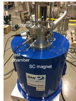
Figure 2: Test bench of ion source.
