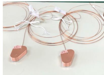
Figure 8: Processed C-H coil.
