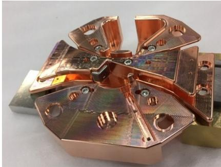
Figure 4: Pre-assembled electrode. This can be included within 100 mm diameter.
