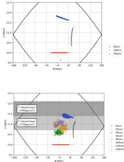
Figure 5: Results of G4BL tracking in longitudinal direction for all 20 turns for MERIT-PoP ring for two different cases; upper and lower graph show the result without and with the internal target, respectively. The two grey regions in the lower graph indicate the position of each stage of the internal target.
