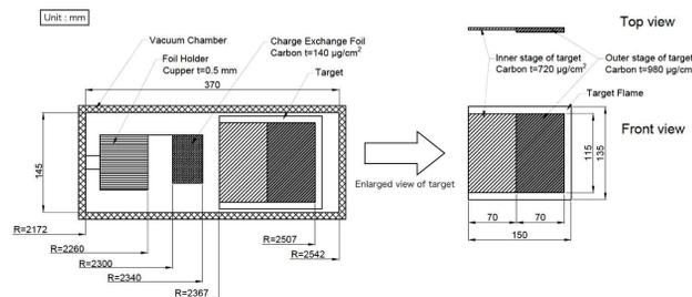
Figure 4: Design of the internal target.
