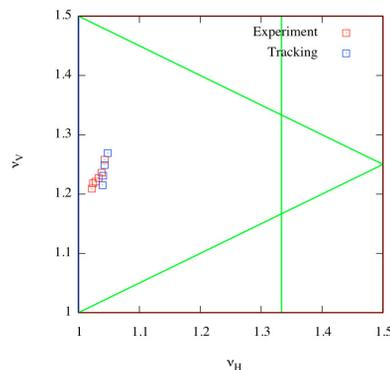
Figure 3: Betatron tune of the MERIT-PoP ring. Red and blue plots show the results of measurement and tracking simulation, respectively. Betatron tunes were measured and calculated by changing the focusing and defocusing magnetic field strength.
