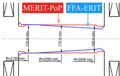
Figure 2: Schematic view on modification of magnetic pole shape. This figure shows the pole shape of focusing magnet of the FFA-ERIT ring and the MERIT-PoP ring, respectively.
