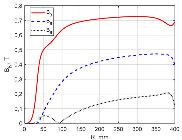
Figure 4: Fourier harmonics of the cyclotron magnetic field.
