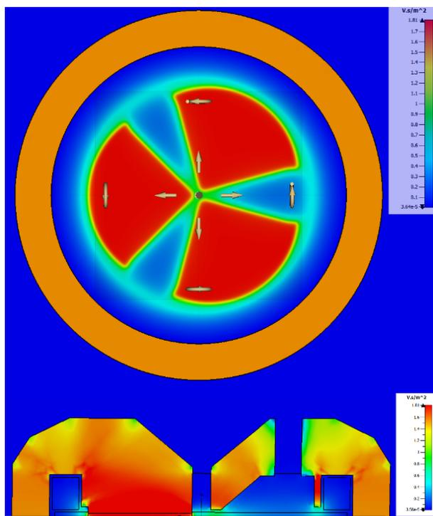
Figure 2: Magnet flux distribution through median plane (up), inside the yoke of the magnet (down).
