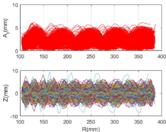
Figure 7: Amplitudes of radial oscillations and vertical motion of the beam during acceleration.
