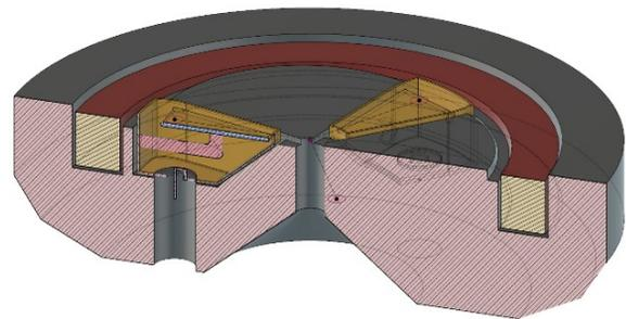
Figure 1: Layout of the 3D computer model of the cyclotron.
