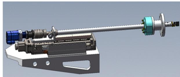
Figure 5: The structure of the movable stripping target.
