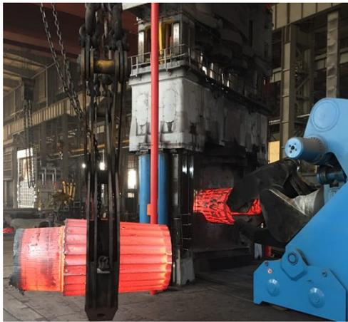
Figure 3: The magnet blank parts are being forged.
