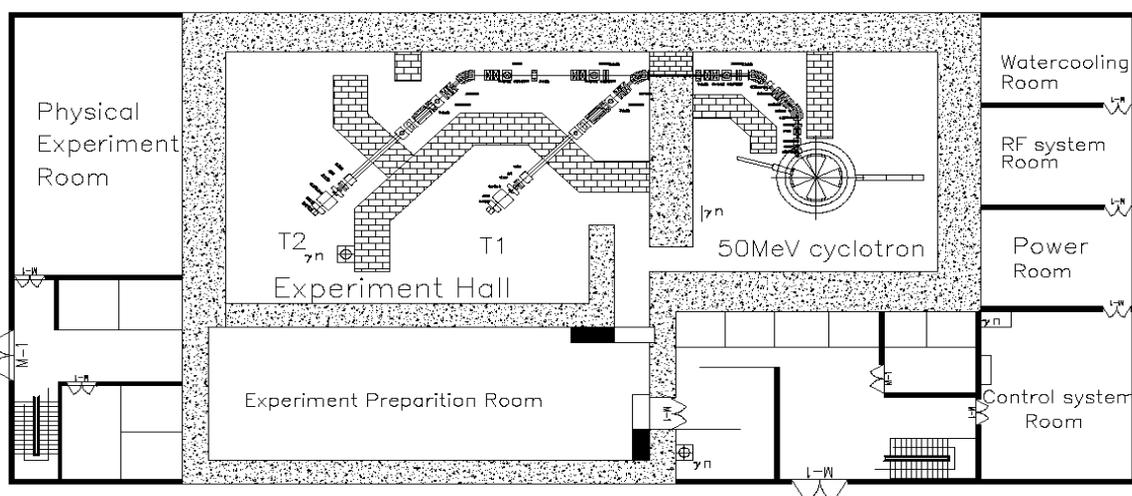
Figure 1: Layout of the proton irradiation facility based on 50 MeV cyclotron.
