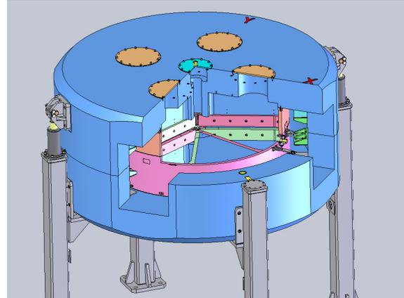
Figure 2: The main magnet of CYCIAE-50.
