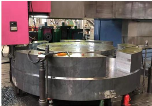
Figure 4: The magnet parts are being machined on a milling machine.
