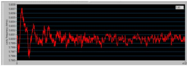
Figure 5: A2C Resonance controller learning process at 5.8 MHz constant resonance point.
