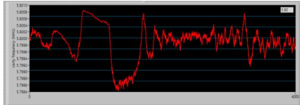
Figure 6: A2C Resonance controller learning process in resonance point shift model.
