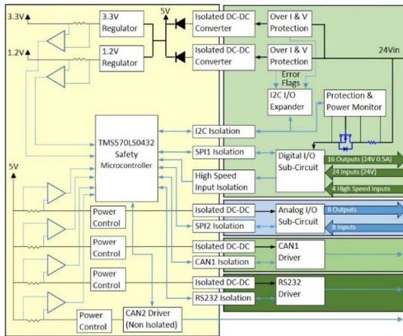
Figure 4: Controller block diagram.
