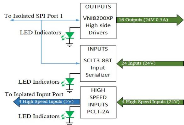
Figure 5: Digital I/O sub-circuit.
