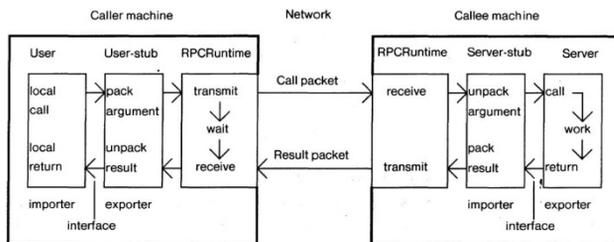
Figure 7: Components of RPC system and their interactions.
