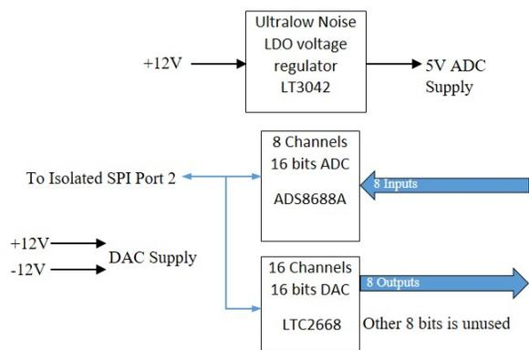
Figure 6: Analog I/O sub-circuit.
