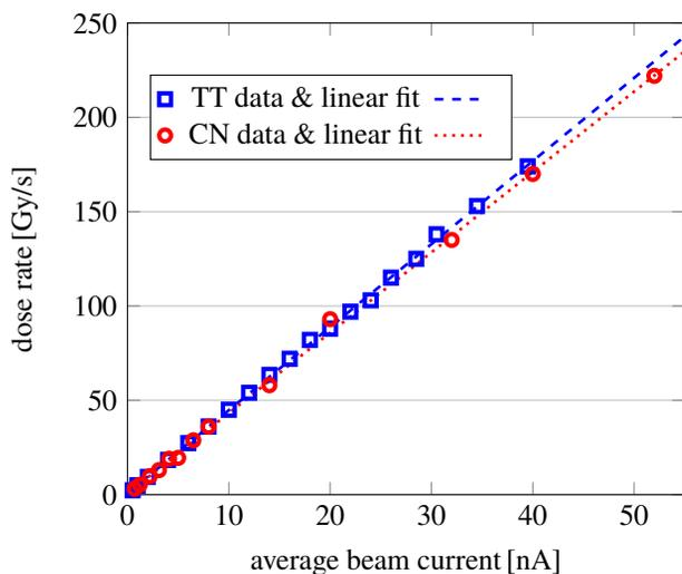
Figure 2: Measured dose rate at the target from each injector.
