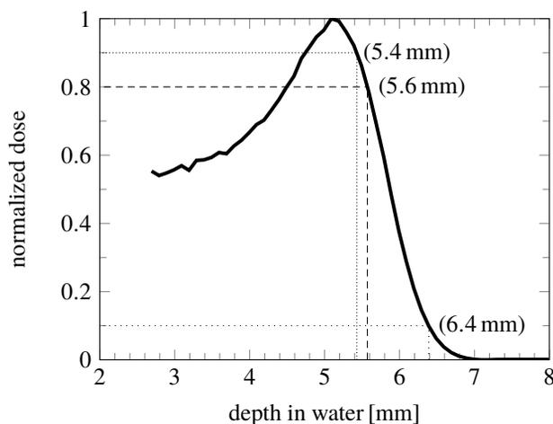
Figure 3: Measured Bragg peak with corresponding distal points in a water phantom for mouse irradiation.
