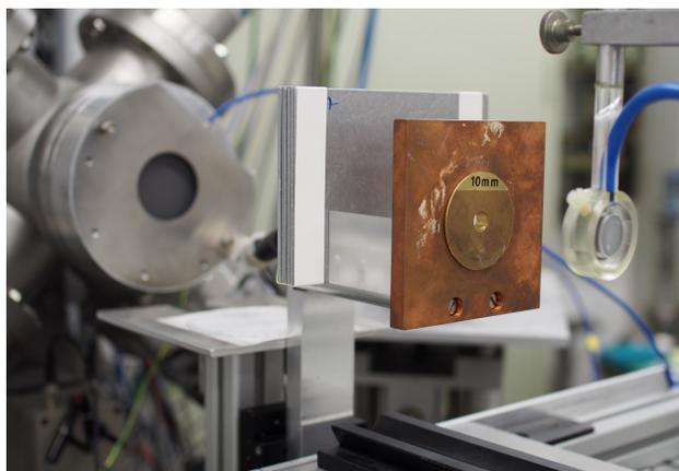
Figure 1: Photo of the experimental setup. The protons travel from left (vacuum beamline exit port) to right (dose monitor with blue cable) in air, while passing through an aluminum plate and a round bronze collimator.
