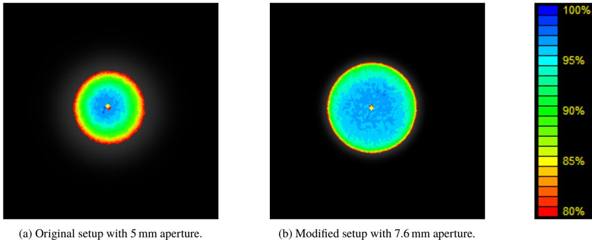
Figure 4: Measured normalized intensity of the transverse beam profiles at the target in grayscale, color-contoured between 80%–100%.
