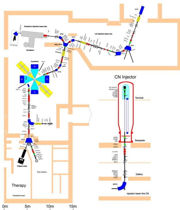
Figure 1: Layout of the accelerators and target stations.
