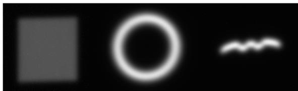
Figure 4: CCD images of the proton beam using the scanning system. Rectangular, circular or irregular shapes are feasible.
