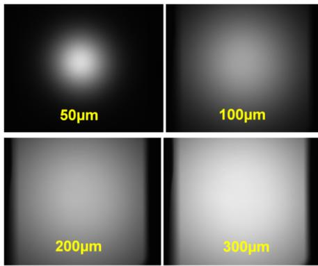
Figure 7: CCD images of the full beam spot using different scattering foils. For 200  $\mu\text{m}$  and 300  $\mu\text{m}$  thickness, the overall beam spot is larger than the entrance aperture of the CCD camera.
