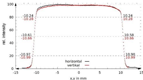
Figure 3: Line scan in x and y of a scanned irradiation field with a quadratic aperture having 20 mm edge length [1].
