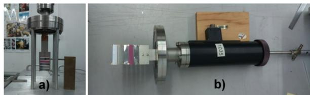
Figure 6: Adjustment unit for positioning of the foils on the beam line axis (a), moving mechanism with three different foils and a ruby quartz.
