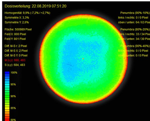
Figure 5: CCD image in false colours of the proton beam using the scattering foil upstream, showing a very homogenous dose distribution.
