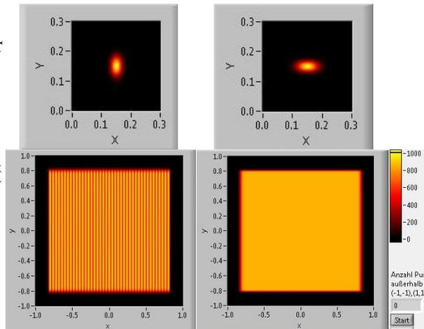
Figure 2: The top row shows two different beam spots used for scanning. The simulated dose distribution for identical settings of the scanner is shown in the lower row.
