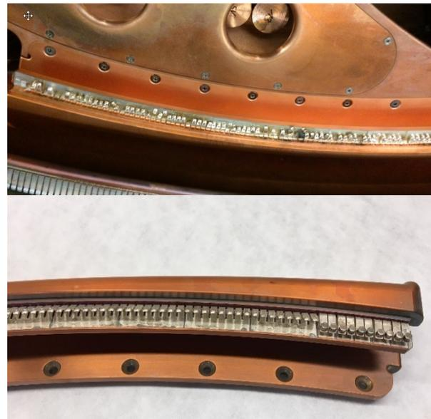
Figure 4: Top: Dee Rim with old design of contact fingers. Starting from the edge of the Dee Rim, the contact fingers are melted due to high currents caused by disbalanced EM fields. Bottom: Dee Rim with new-designed contact fingers. No sign of deterioration is noticeable. Note, that this Dee Rim was installed during RF and beam commissioning.
