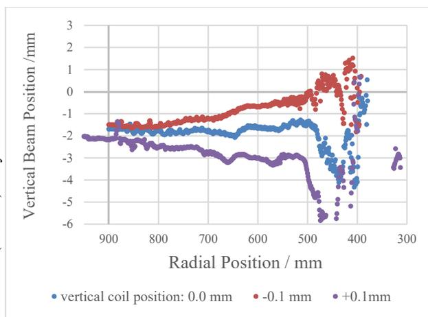
Figure 6: Vertical beam oscillation along cyclotron radius for 3 different vertical coil positions (please note: radial position axis is inverted, 360 mm corresponds to outermost radius/ extraction).
