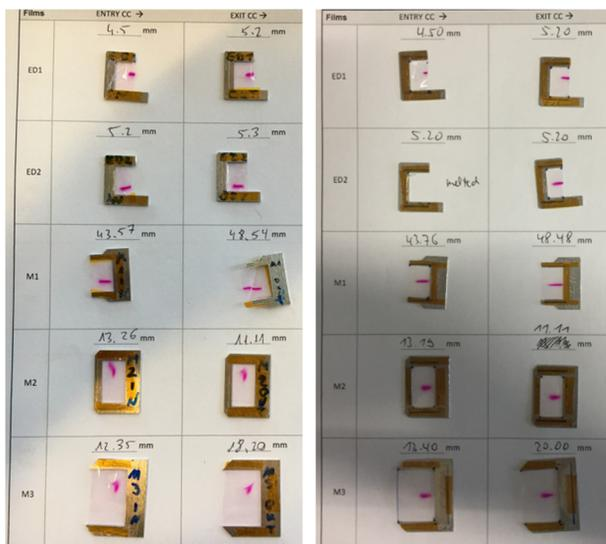
Figure 5: Examples of foil irradiations performed during beam commissioning. Left: vertical beam oscillations are visible along the beam path due to misaligned (tilted) coil. Right: coil pre-alignment eliminates oscillation and allow an straight beam path through the extraction.
