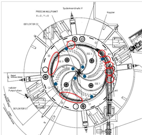
Figure 3: Sketch of cyclotron layout. The red circles depict the extraction element positions (see Fig. 5).
