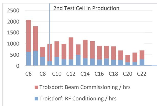
Figure 2: Used working hours for RF and beam commissioning in the Troisdorf cyclotron test cells.
