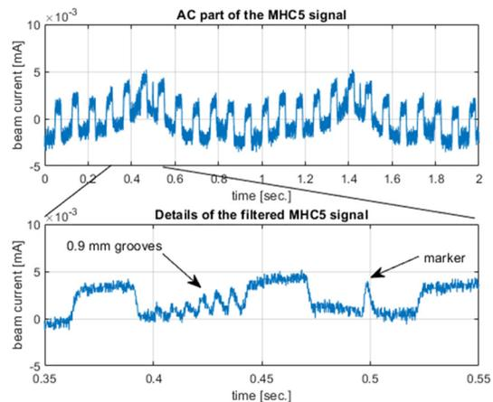
Figure 4: Example of modulations for off-axis position.
