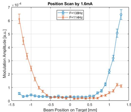
Figure 5: 114 Hz and 138 Hz spectral lines as function of the beam position on the target.
