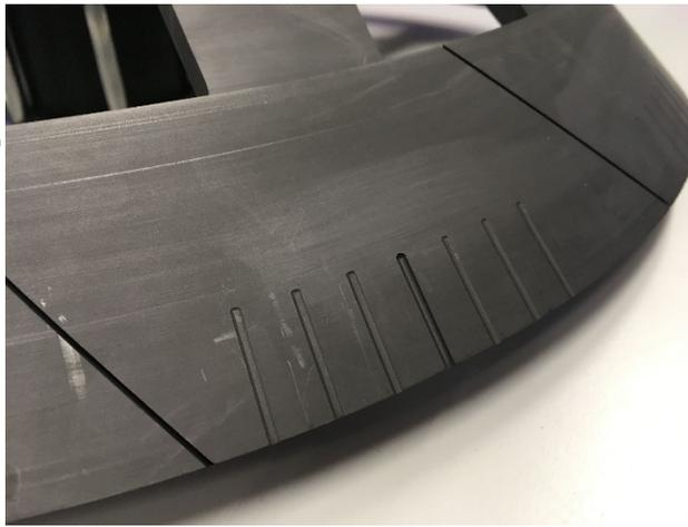
Figure 2: Detail of a segment showing the grooves. On that particular segment the middle groove is milled 1 mm deep (the other grooves of this segment are 0.3 mm deep). This groove acts as absolute marker.
