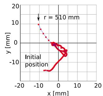
(c) Centered beam with the field bump at azimuth  $98^\circ$ .
