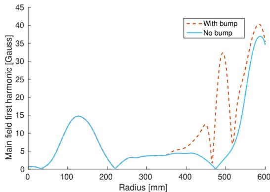
Figure 3: First harmonic introduced by the magnetic field bumper at proton regime for 28 MeV.
