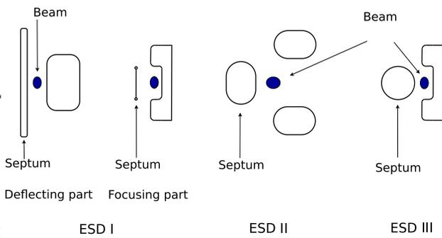
Figure 2: Electrostatic deflectors profiles. Not labeled profiles belongs to high voltages electrodes.
