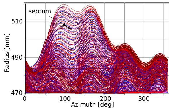
Figure 6: Orbit separation at azimuth  $110^\circ$  by a magnetic field bump and ESD septum position.
