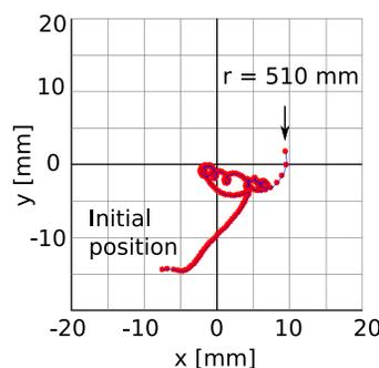
(b) Centered beam with outer harmonic coils. Center shifts to azimuth  $\sim 70^\circ$ .
