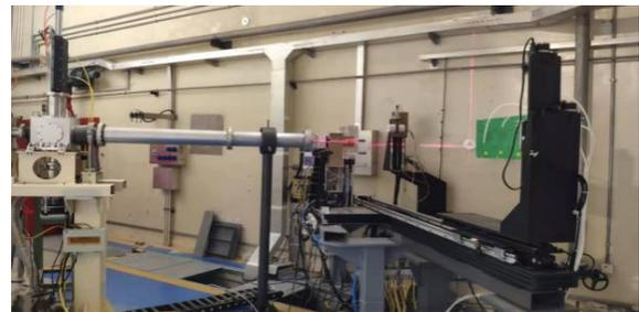
Figure 1: Beam line and experimental terminal of single-event effect.
